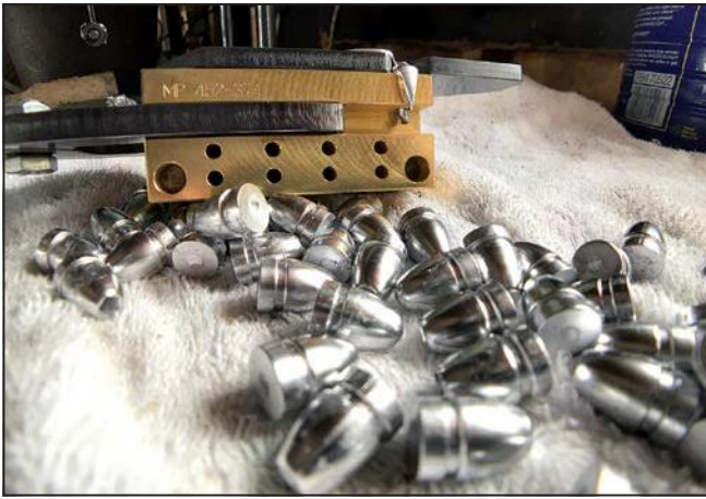
MP four-cavity brass moulds are big and require preheating and casting a few times to bring them up to the correct temperature to produce fully formed bullets.
