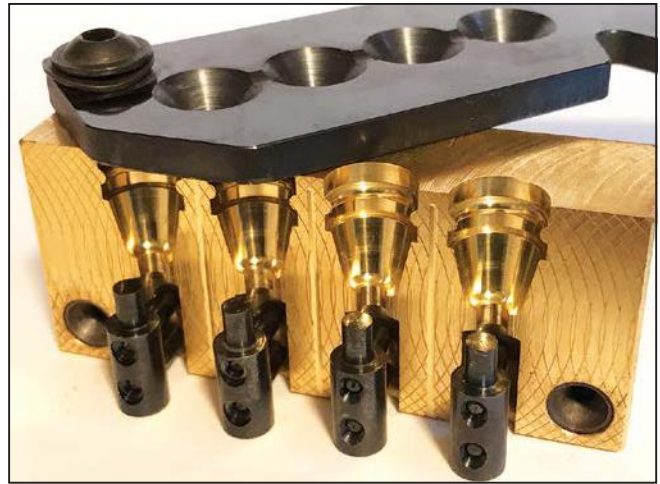
Many moulds come with pins to cast different types of bullets. The pins attach to screws that slide in and out of the cavities.
